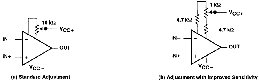
Figure 44. Input Offset Voltage Nulling Circuits
